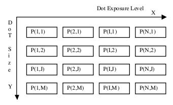
Figure 1. Illustration of Dot formation Chart. Each patch P(I,J) represents a dot formation at specific dot size and dot exposure.
